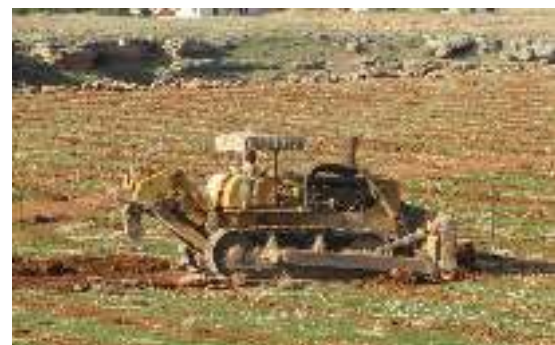
Figure 6-1. Soil preparation of the Maqne site - photo shows the ripper used to remove the surface rocks and expose soil underneath. The pattern created is inevitably less random than with other techniques
